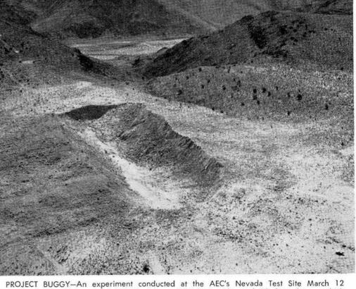
produced this ditch - about 900 feet long, 300 feet wide, and 80 feet deep - which resulted from the simultaneous underground detonation of five nuclear explosives. The ditch is three times as long as a football field and more than twice as wide. An eight-story building would stand upright in it. The experiment was conducted as part of the AEC's Plowshare program in which excavation technology is being developed for peaceful purposes. A number of Sandians participated in the project.
